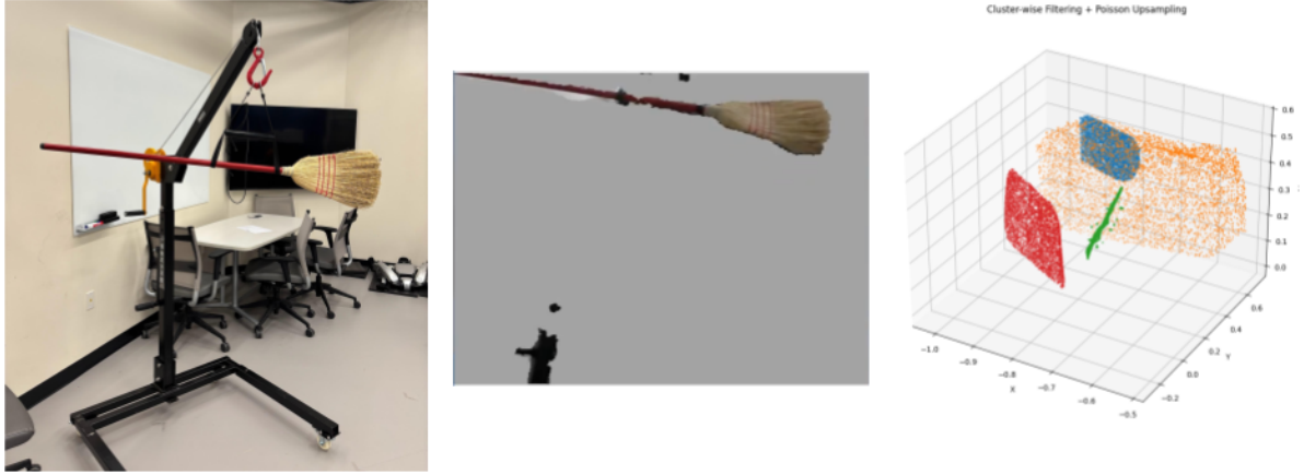
Figure 3.9: Suspended broom used as an overhead obstacle during indoor trials. The obstacle height was approximately 4 ft 2 in.
